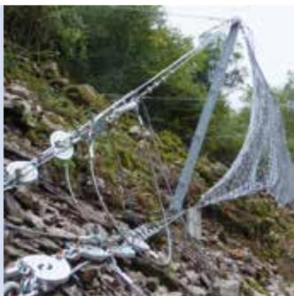
The certification test for the ISOSTOP E series was performed at the Swiss federal rockfall test facility in Walenstadt. The tests were carried out by the WSL. The product certification was accomplished by the independent and officially authorized construction building and testing and research Institute TSUS.
